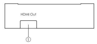
(1). HDMI Out: This slot is to connect with LCD TV or HD monitor for both video and audio display with HDMI cable.
